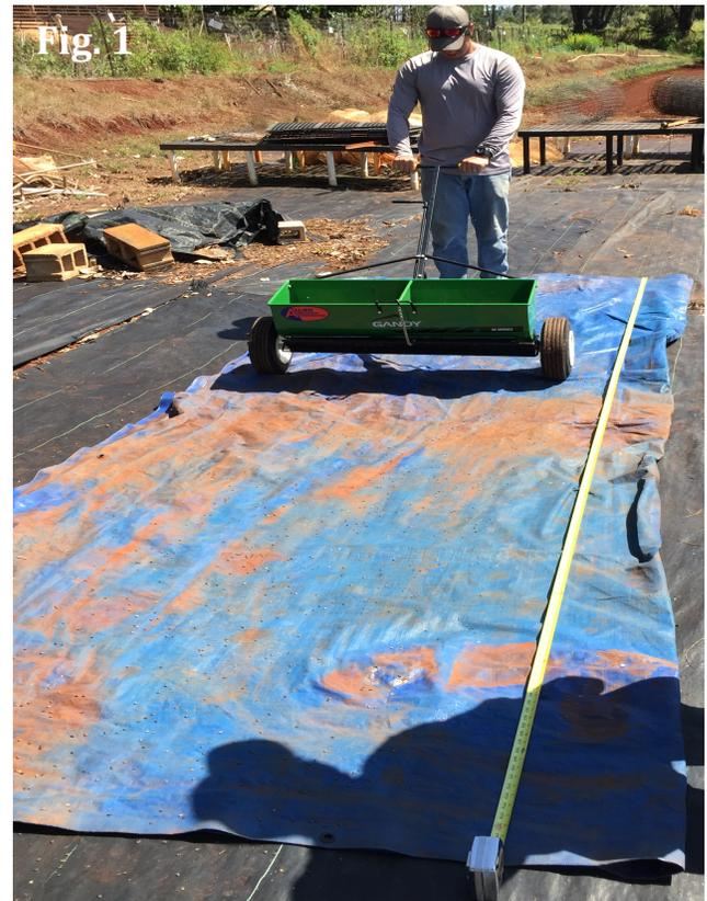
**Step 1:** Measure the test area equal to 1/160<sup>th</sup> of an acre (272 sq ft) on a weed mat or tarp larger than the width of the spreader (Fig. 1). For example, the dimension of the calibration area can be 91 ft by 3 ft or 136 ft by 2 ft.
