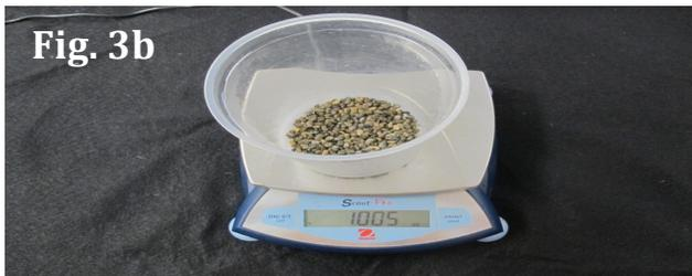
**Step 3:** Collect and weigh total amount of seeds or granular fertilizer dropped over the measured area (Fig. 3a, b).
